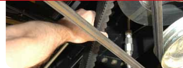
Check the tension of all belts and chains at the start of each day.
