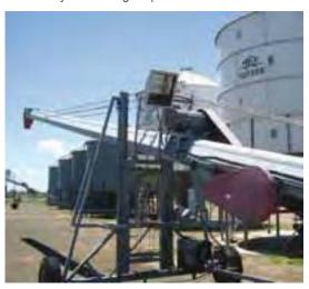
Ensure that all auger flights, engine pulleys, drive belts and shafts are properly guarded and that the guards are in good condition before using all augers.
